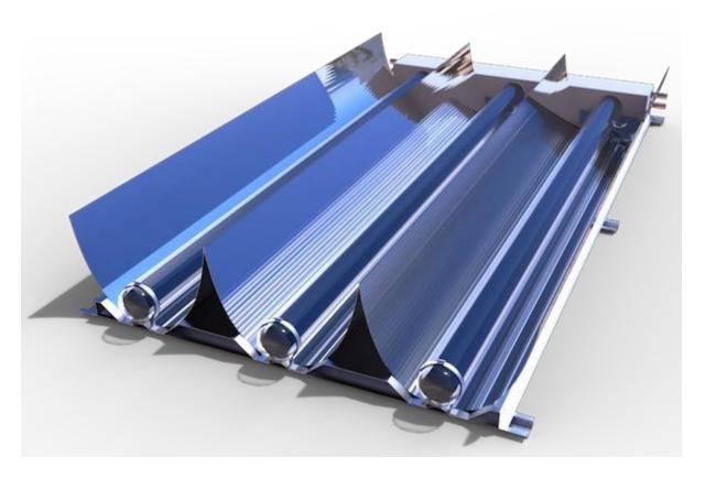
XCPC or External Concentrating Parabolic Collector is the new technology in the market, manufactured by Artic Solar in Jacksonville, Florida. The patented XCPC Non-Imaging Concentrating Collector is a non-tracking high temperature collector capable of +350oF temperatures for SIPH applications and more importantly for Advanced HP integrated Desalination systems as demonstrated by WaterFX for cleaning up subsurface agricultural waste water in California. (Pilot demonstration of concentrated
