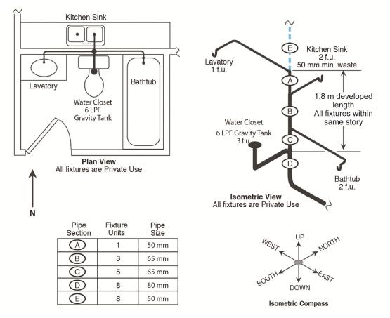
Figure 908.1a Wet Vent Sizing Example 1
