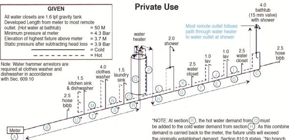
Hose Bibb sizing. Each pipe section serving only one hose bibb is assigned a fixture unit value of 2.5. Section B serves one hose bibb with a rating of 2.5 plus one "additional" hose bibb with a fixture unit value 1.0. The total hose bibb fixture unit value at section B is 3.5. See Note 8 at bottom of Table 610.3
